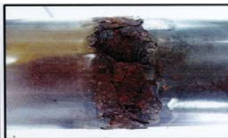
HVOF can be used to repair OD surface pitting
