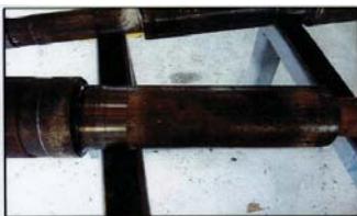
HVOF can be used to repair OD surface pitting
