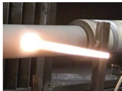
Twin Wire Arc Spray and final machining to repair a damaged Kelly Mandrel
